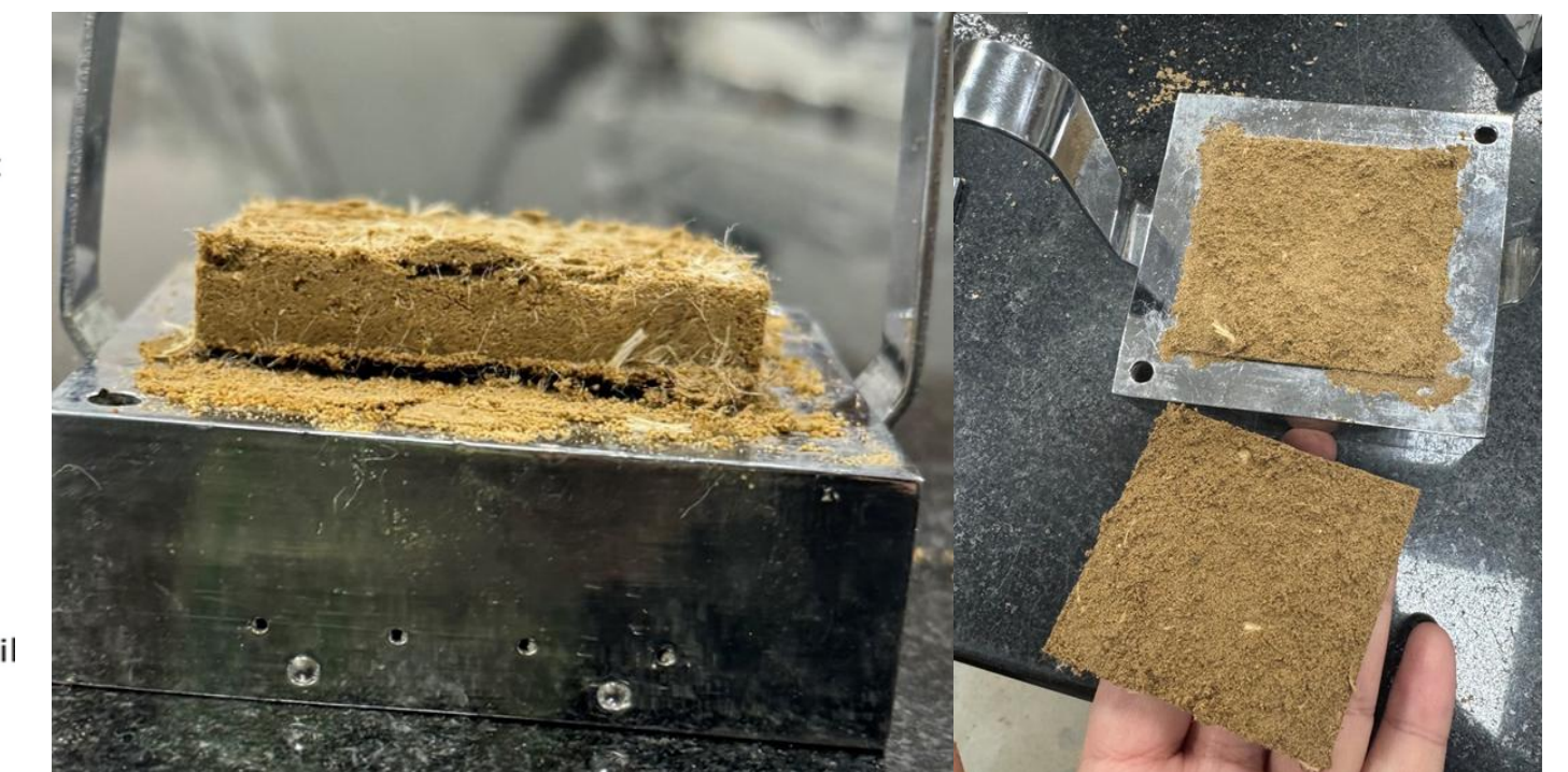
Fig:- PP fiber- soil interaction after shear test showing bridging and interlocking along the failure plane
